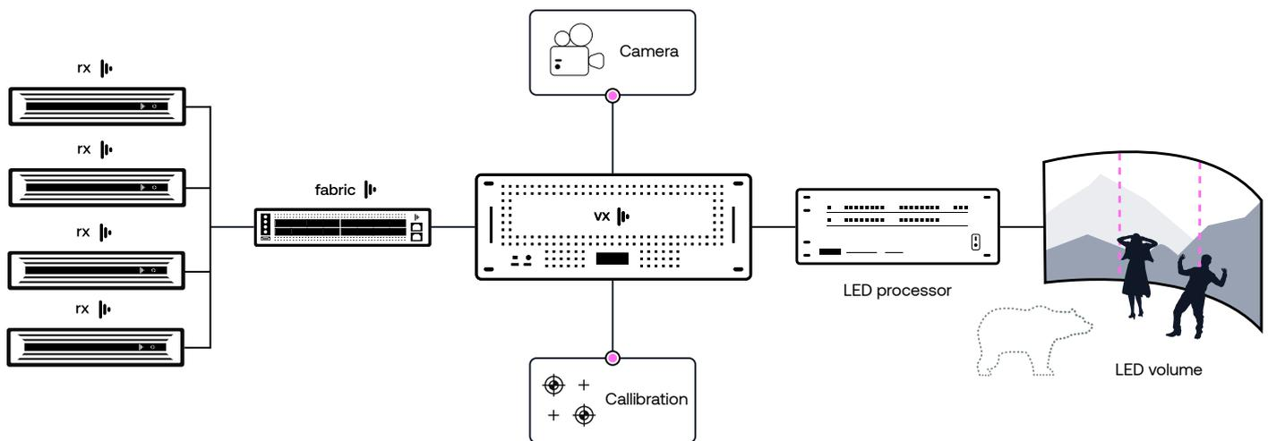
*Render nodes can be used to scale content endlessly - rendering them across different surfaces including projection canvases and LED screens.*
